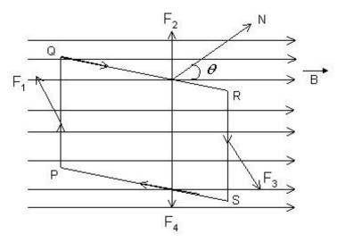
Sides PQ and RS of the current loop are perpendicular to  $\,\mathrm{B}$ ; therefore, the magnitude of each of the forces  $\,\mathrm{F_1}$  and  $\,\mathrm{F_3}$  is
