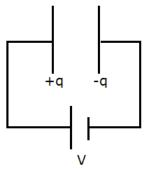
For a parallel plate capacitor (with vacuum between the where A is the area of each plate and d the separation between them)
